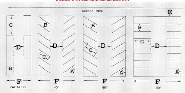
FIGURE 12-4A PARKING STALL AND AISLE LAYOUT
