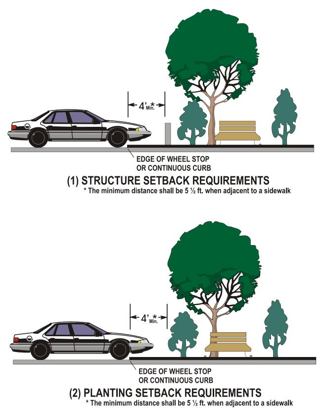
FIGURE 12-4D PAVEMENT AREA ADJUSTMENT WITH CONTINUOUS CURB USAGE
