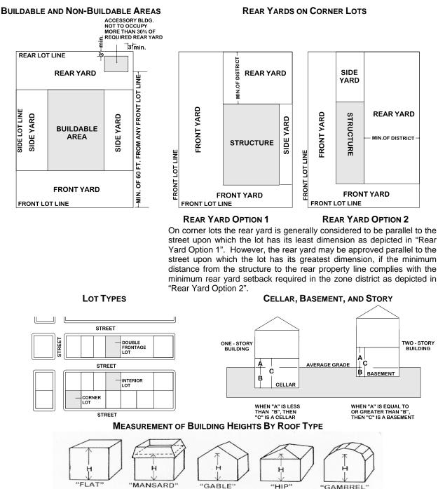
Building Height is measured as the vertical distance from the average grade to the highest point of the coping of a flat roof or to the deck of a mansard roof, or to the mean height level between eaves and ridge for gable, hip and gambrel roofs excluding elevator shafts, chimneys and other structures.
